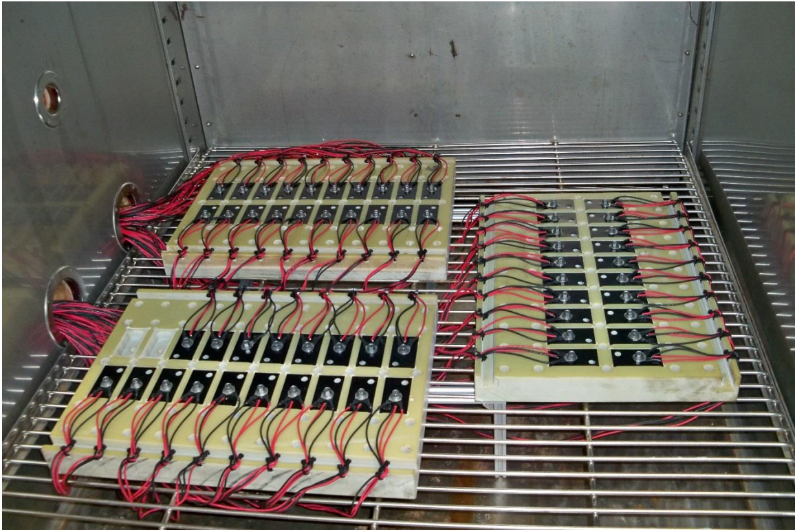
Temperature/Humidity, Samples 1 to 58, Test Setup
